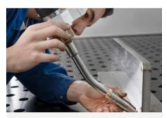
Simple programming: With the free-drive function, the cobot is shown by hand where to weld - including intermediate waypoints and sections.
